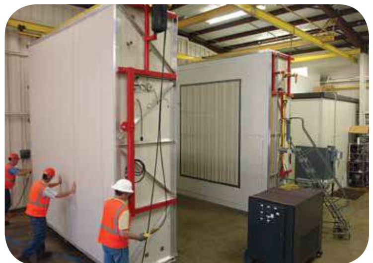
The Butler® Guarded Hot Box can test actual 8'X10' roof or wall sections, assembled just as they would be on your building to provide extremely accurate estimates of your building's heating and cooling energy consumption.
